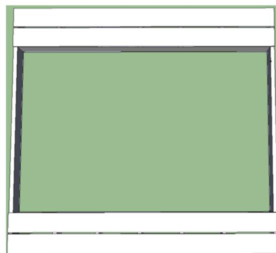
**Step 6:** Create the bench bottom. Lay two 1x8x8' pieces parallel to one another, spaced 1/2" apart. Lay the 2x6x15 1/2" perpendicular to the boards, offset 1 1/2" from the edge of the end of the 1x8. Attach using the 2 1/2 deck screws. Attach the second 2x6x15 1/2 to the inside of the first 2x6x15 1/2". Repeat this step again to make a second bench bottom for the other side of the sandbox.
