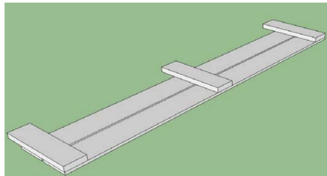
**Step 9:** Attach the bench back. Lay the bench pieces you created in step 8 parallel to the bench bottom, spaced 1/2" away, with the 2x6's on the top side. Attach with three **hinges** per side, this time on the **bottom** side.
