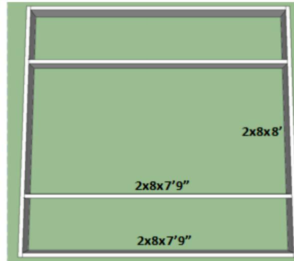
**Step 4:** Next, add support joists. Attach the 2x8x12 1/2" pieces running perpendicular in between the two 2x8x7'9" pieces (5 per side). They should be spaced at approximately 1'3" on center. (Note: 1'3" is an approximation. Do your best to space evenly). Attach using the 2 1/2in deck screws.
