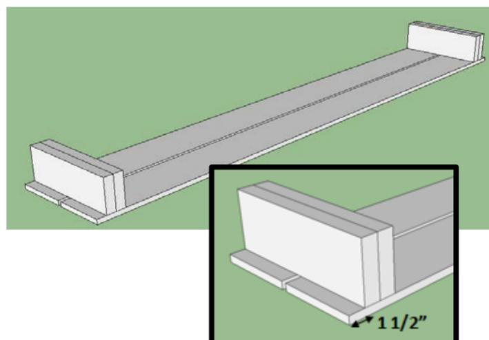
**Step 7:** Attach the bench bottom. Lay the bench piece you created in step 6 parallel to the first two lid pieces, spaced 1/2" away, with the 2x6's on the bottom side. Attach with three **hinges** (per side) on the top of the sandbox.
