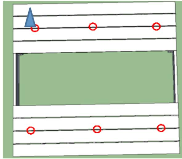
**Step 8:** Create the bench back. Lay two 1x8x8' pieces parallel to one another, spaced 1/2" apart. Lay two 2x6x20-1/2" (per side) perpendicular to the boards, flush with the edge and one corner. The 2x6s will extend past the edge at the 1x8 corner. The third 2x6x20-1/2" should be flush with the top and centered in the middle of the 1x8x8'. Attach using the **2in deck screws**. Complete this step twice.
