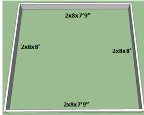
**Step 3:** Attach the inside frame supports. Run your remaining two 2x8x7'-9" pieces parallel to the 2x8x7'9" already in place. Be sure there is 12 1/2" between the boards. (Hint, use one of your 2x8x12 1/2" pieces as a spacer.) Attach using 2 1/2in deck screws.
